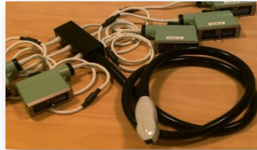
32 x 32 = 1024 element Matrix Probe from Vernon
