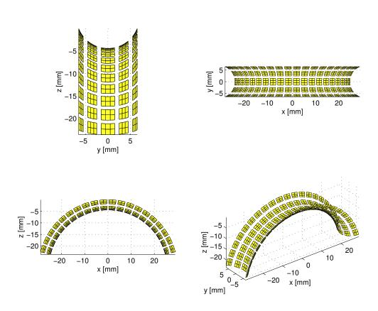
Figure 3.13: Elevation focused convex array transducer with element division in the elevation direction. The curvature in the elevation direction is exaggerated in the figure for illustration purposes
