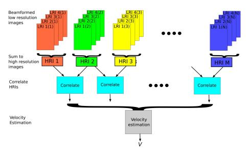
Fig. 3. Traditional SA sequence for velocity estimation. HRIs are created in blocks making the effective  $f_{prf,eff}$  low. LRI 1(2) denotes LRI for emission 1 in high-resolution sequence 2 (first emission in the green block).
