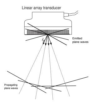
Figure 5.21: Plane wave imaging.
