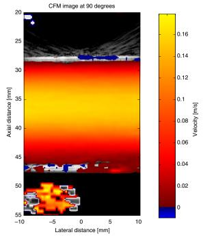
Fig. 9. Synthetic aperture color flow map image of flow rig data at a  $90^{\circ}$  flow angle obtained using 128 emissions (from [38]). (For interpretation of the references in color in this figure legend, the reader is referred to the web version of this article.)
