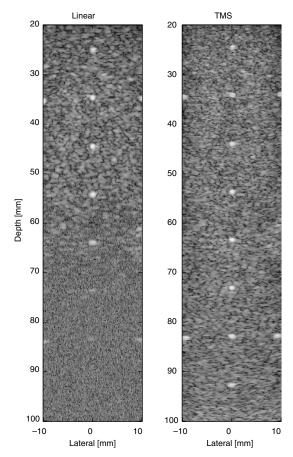
Fig. 4. Measured linear array image (left) and TMS image (right) on a multi-target phantom with 0.5 dB/(cm MHz) attenuation. The scanned section contains twisted nylon wires spaced axially by 1 cm throughout the imaged region. The dynamic range in the images is 50 dB (from [32]).
