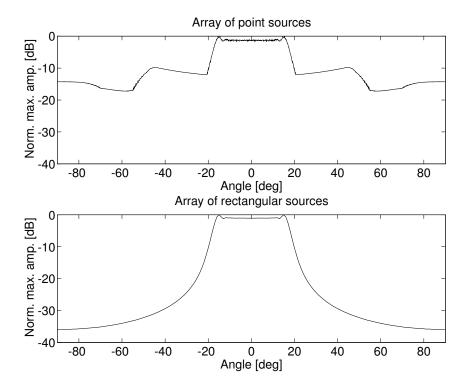
Figure 3.6: Beam profiles for an array consisting of point sources (top) or rectangular elements (bottom). The excitation pulse has a frequency of 3 MHz and the element spacing is 1 mm. The distance to the field point is 100 mm (from [9], Copyright Cambridge University Press).
