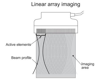
Figure 3.8: Linear array transducer for obtaining a rectangular cross-sectional image.
