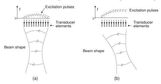
Figure 3.9: Electronic focusing and steering of an ultrasound beam.
