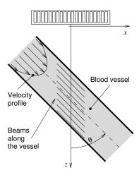
Figure 5.17: Directional beamforming along the flow lines (from [96]).
