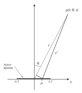
Figure 3.1: Geometry for line aperture.
