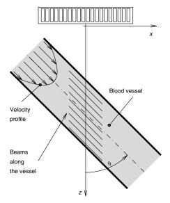
Fig. 7. Beamforming is made along the laminar flow (from [38]).
