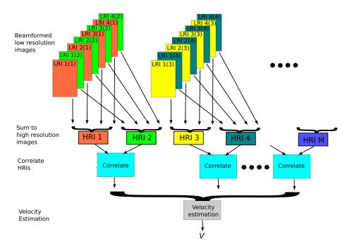
Fig. 4. Interleaved SA sequence where LRIs are repeated to minimize the distance between HRIs. The same colored LRIs are summed to yield one HRI. The effective  $f_{prf,eff}$  is equal to the highest possible value due to the interleaving. Correlations in the blue boxes yield the same correlation function, which are then averaged to improve precision.
