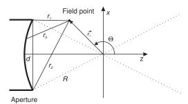
Figure 2.11: Definition of variables for spatial impulse response of concave transducer.
