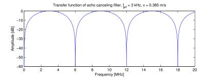
Figure 5.6: Transfer function of echo canceling filter.
