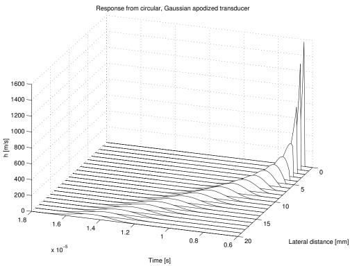
Figure 2.15: Spatial impulse response from a circular aperture. Graphs are shown without apodization of the aperture (top) and with a Gaussian apodization function (bottom). The radius of the aperture is 5 mm and the field is calculated 10 mm from the transducer surface.
