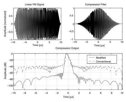
Fig. 3. Top left: Modified linear FM signal with a 7 MHz center frequency and 7 MHz bandwidth. A Tukey window with a duration of 10% has been applied. Top right: Modified compression filter using a Chebychev window with 70 dB relative side-lobe attenuation. Bottom: Compression output for the conventional FM signal (dashed) and the modified FM signal (solid). The effect of a linear array transducer has been introduced in the compression outputs (from [32]).
