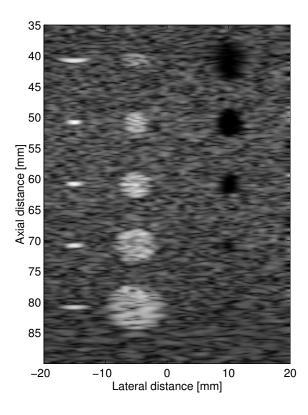
Figure 3.17: Computer phantom with point targets, cyst regions, and strongly reflecting regions.
