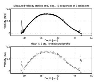
Fig. 8. Estimated profiles from the flow rig at a 90° flow angle. The top graph shows 20 independent profiles estimated and the bottom graph shows the mean profile (solid line)  $\pm$  3 standard deviations (dashed lines). From [38].
