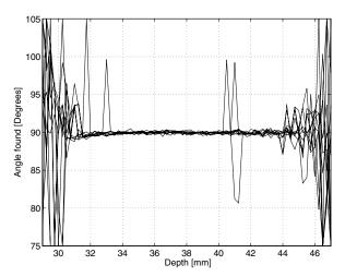
Fig. 12. Estimated velocity angles for a true velocity angle of  $90^{\circ}$  (from [40]).
