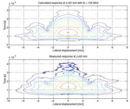
Point spread function for concave, focused transducer
