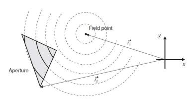
Intersection of spherical waves from the field point by the aperture, when the field point is projected onto the plane of the aperture
