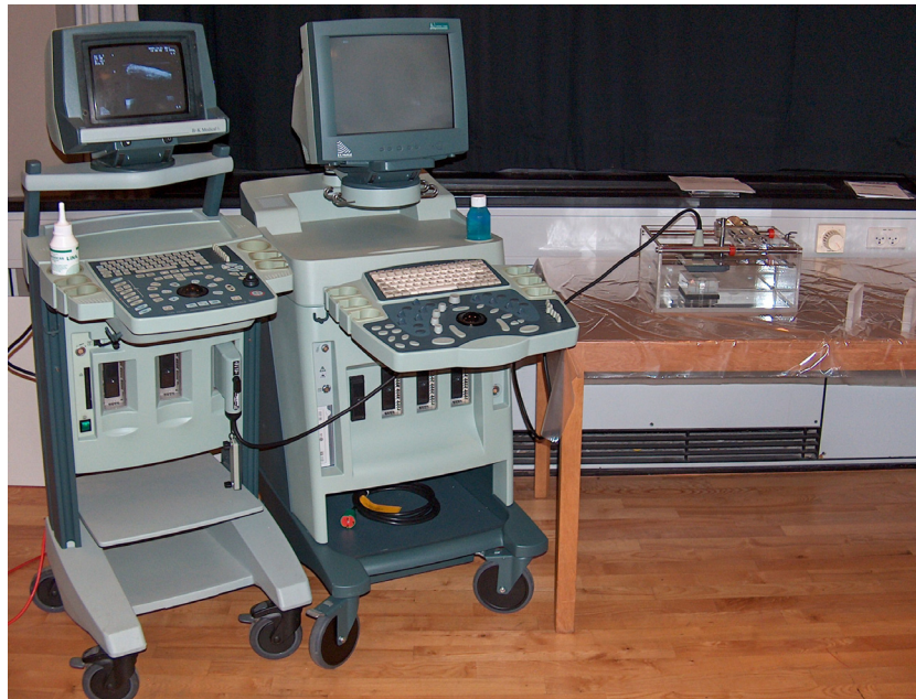
Figur 2 The entire setup for ultrasound recording, here shown with two different ultrasound scanners. The one to the left is a 2102 Hawk while the one to the right is a Viking 2400. The latter is used in the ultrasound measurements.
